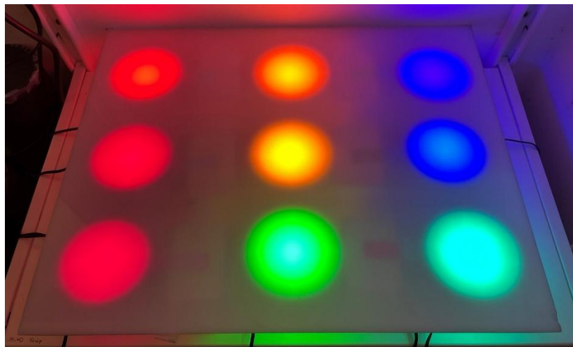
Figure 1. Home-built cultivation bench with nine different monochromatic growth lights from 430 to 690 nm.
