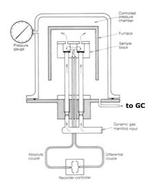
The concept behind evolved gas analysis is that the study of unknown materials and/or thermal processes is much easier if we also use a detector to selectively identify released compounds the byproducts (volatiles, combustion products, etc.). This can be done by coupling the gas output of a TG or DTA instrument to a selective detector, such as a spectrometer or a gas chromatograph. exemplyfied in the schematic on the left for a DTA-GC combination.
