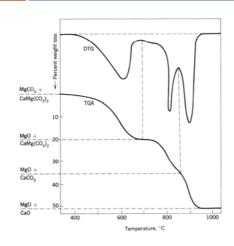
It is very useful to record the first derivative of the TG/TGA curve (DTG) also, because it makes the noticing small features/boulders on the curve much easier (they appear as peaks).
