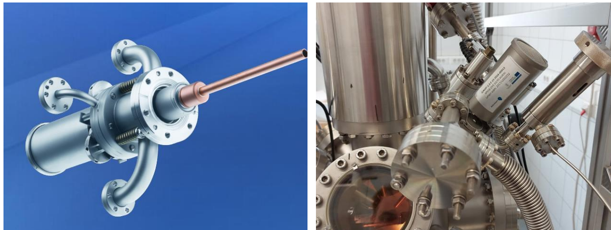
Schematic view of the SPECS UVS 10/35 lamp and after the installation in the SPECS XPS
