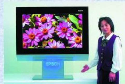
2004 EPSON a screen of 4 blocs of 20" each
