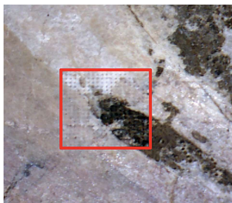
Figure 1. Optical Image of bastnäsite mineral used for LIBS analysis. Tan region = bastnäsite and white region = barite.
