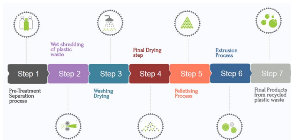
Figure 2. Stages of mechanical recycling process for plastic waste [8]
