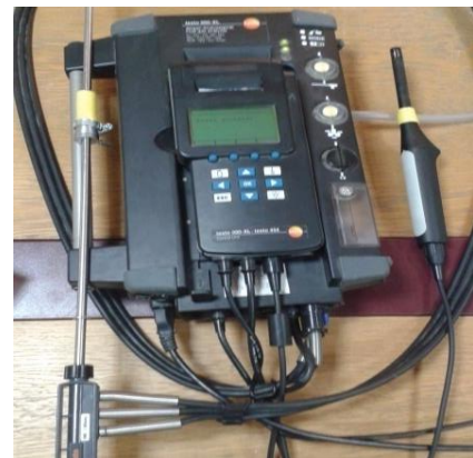
Figure 2. Testo 350XL analyzer
