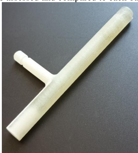
Figure 1. 3D-printed plastic V-groove nebulizer
