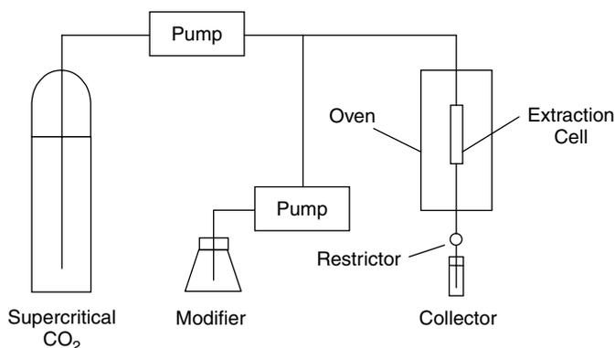
Figure 3.6. Schematic diagram of an off-line SFE system.
