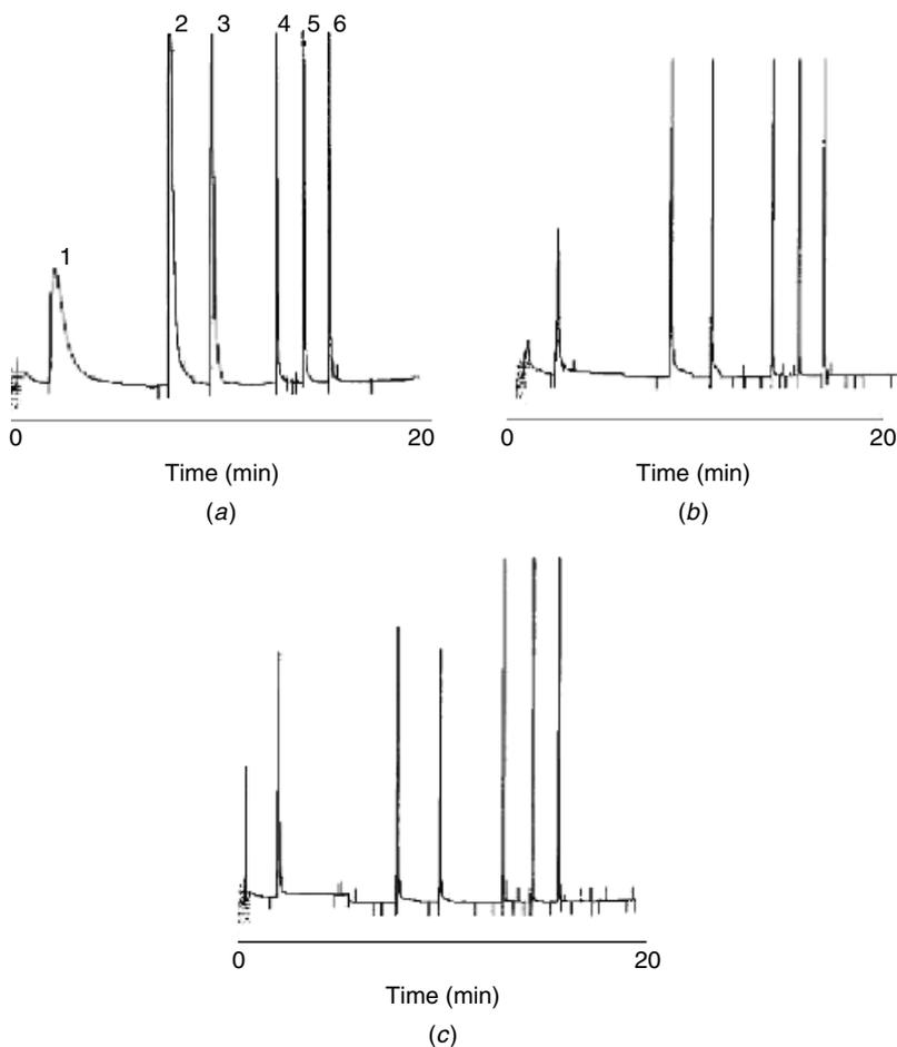
**Figure 4.12.** Effect of inlet liner diameter on SPME injection of hydrocarbons. (a) 4-mm-diameter liner; (b) 2-mm-diameter liner; (c) 0.75-mm-diameter liner. Analytes: 1, octane; 2, decane; 3, undecane; 4, tridecane; 5, tetradecane; 6, pentadecane. [Reprinted with permission from Ref. 44 (Fig. 3). Copyright Advanstar Communications.]
