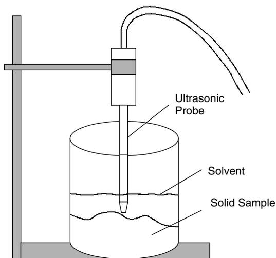
Figure 3.3. Schematic diagram of an ultrasonic extraction device.
