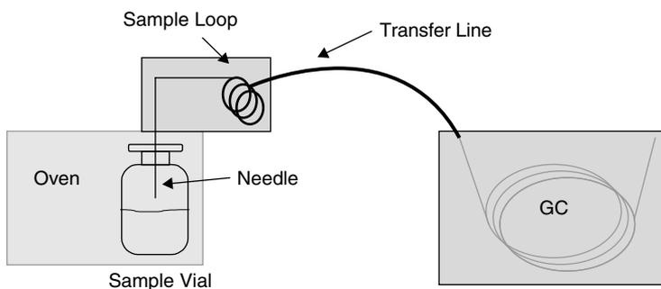
**Figure 4.2.** Schematic diagram of headspace extraction autosampler and GC instrument.
