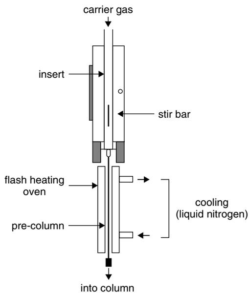
**Figure 2.54.** Schematic representation of the desorption unit. (Reprinted with permission from Ref. 145. Copyright © 2001 American Chemical Society.)
