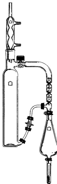
**Figure 2.15.** Continuous liquid–liquid extraction apparatus designed for samples where the extracting solvent is heavier than water in which both extraction and concentration are performed with the same apparatus. (Reprinted with permission from Ref. 46. Copyright © 2002 Kimble/Kontes.)
