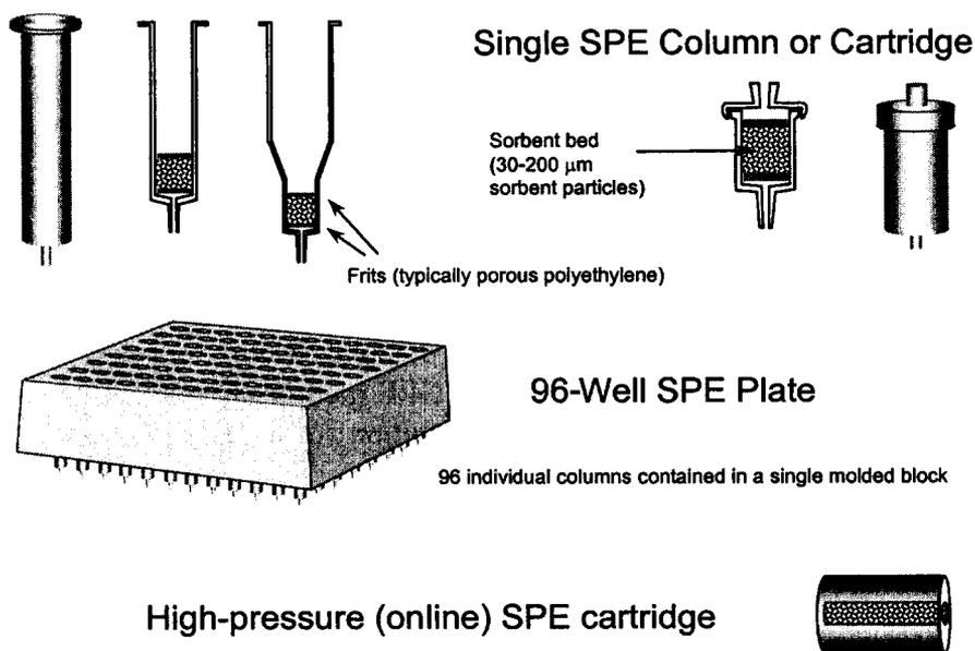
PVDF body (I.D. 1-3 mm), containing 20-40 mg of sorbent between two steel frits
