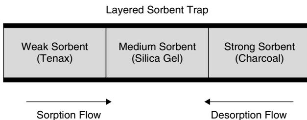
Figure 4.9. Schematic diagram of a multilayer sorbent trap.
