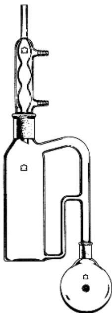
**Figure 2.14.** Continuous liquid-liquid extraction apparatus designed for samples where the extracting solvent is heavier than water. (Reprinted with permission from Ref. 46. Copyright © 2002 Kimble/Kontes.)
