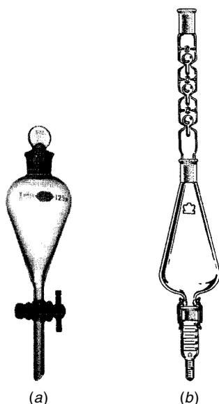
**Figure 2.13.** Liquid-liquid extraction apparatus: (a) separatory funnel and (b) evaporative Kuderna-Danish sample concentrator. (Reprinted with permission from Ref. 46. Copyright © 2002 Kimble/Kontes.)
