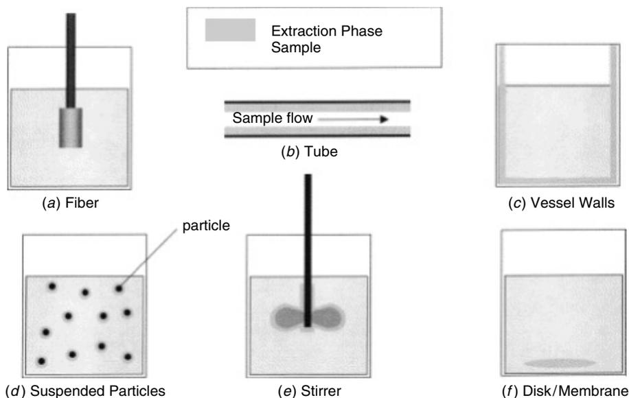
**Figure 2.46.** Configurations of solid-phase microextraction: (a) fiber, (b) tube, (c) vessel walls, (d) suspended particles, (e) stirrer, and (f) disk/membrane. (Reprinted with permission from Ref. 51. Copyright © 2000 Elsevier Science.)
