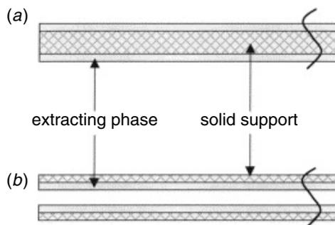
**Figure 2.47.** Two different implementations of the SPME technique: (a) polymer coated on outer surface of fiber; (b) polymer coated on internal surface of capillary tube. (Reprinted with permission from Ref. 51. Copyright © 2000 Elsevier Science.)
