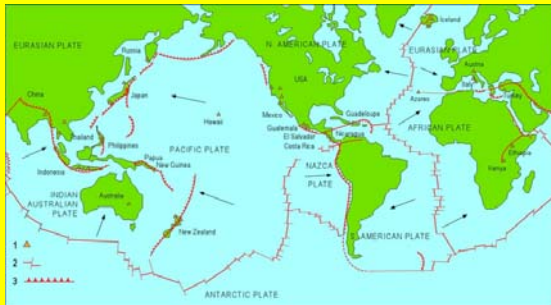
Lithospheric plates, oceanic ridges, oceanic trenches, subduction zones, and geothermal fields. Arrows: direction of plate movement. 1- geothermal fields producing electricity and country name; 2- mid-oceanic ridges; 3- subduction zones (from Dickson and Fanelli, 2004).
