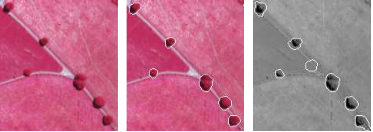
Figure 7: From left to right: a CIR image © IFN; result with multispectral GOC model; result with model in Thesis 2 using only the infrared spectral band;
