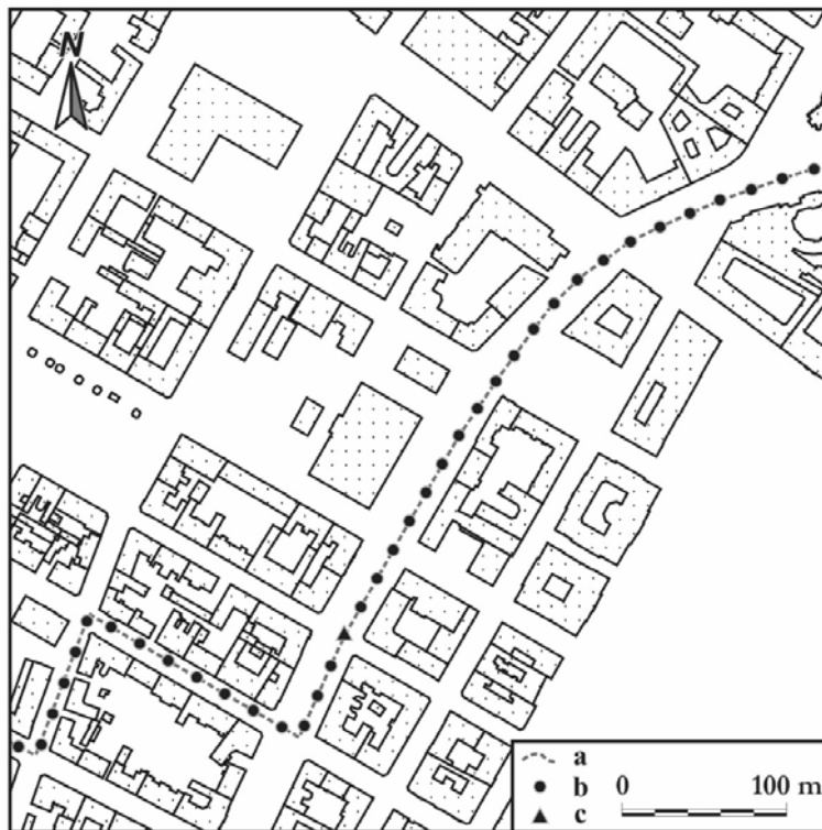
Figure 10 Building plan areas data in a selected part of the city with a section of the measurement route (a – temperature and SVF measurement route, b – SVF measurement points, c – site of the measurement point in Figure 11)
