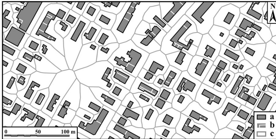
Fig. 5. Lot area polygons (units) in a part of the study area in Szeged, as an example (a: building blocks, b: border of the building footprint within the building block, and c: lot area polygons).
