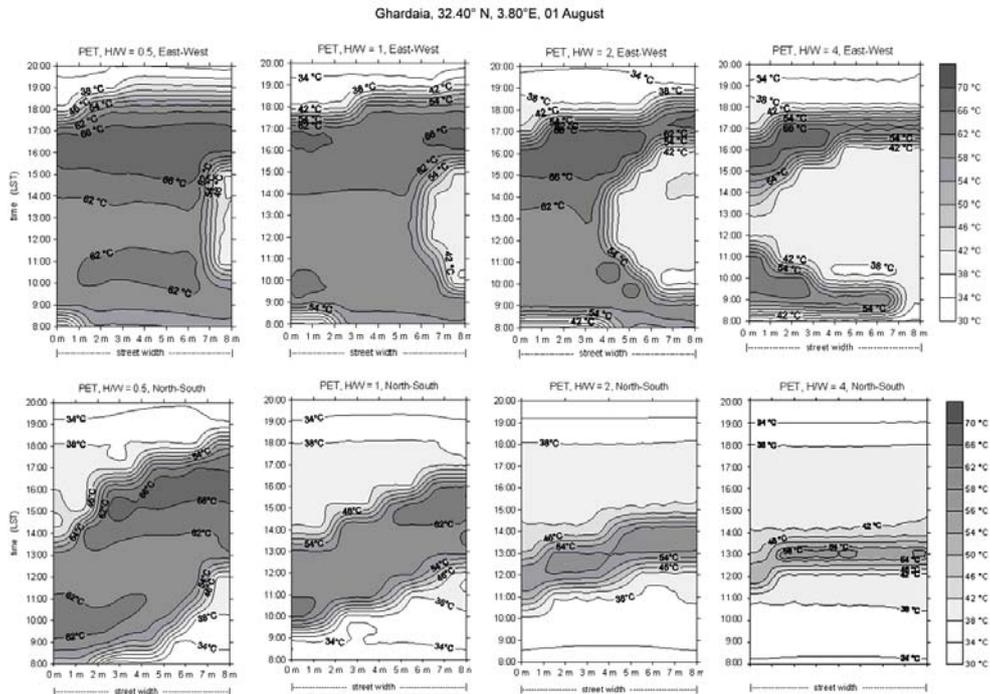
Figure 3 Spatial and temporal distribution of the thermal index PET at street level in urban canyons with aspect ratios H/W from 0.5 to 4 and for E-W and N-S orientations, typical summer day (1<sup>st</sup> August) in Ghardaia, Algeria (32.40° N, 3.80° E)
