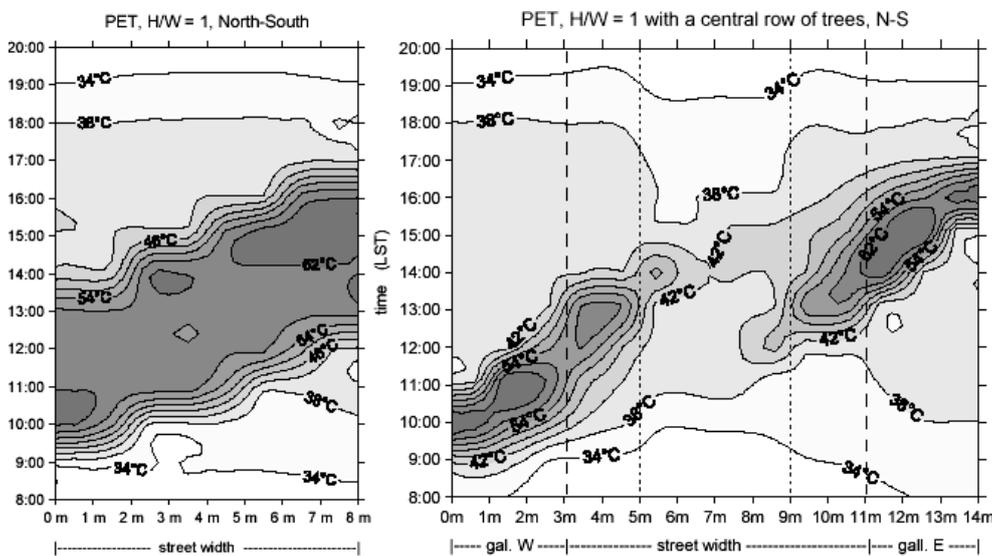
*Figure 5* PET at street level in an urban canyon oriented N-S ( $H/W = 1$ ) with and without trees and galleries (---- footprint of the central planted area; --- footprint of the galleries), typical summer day (1<sup>st</sup> August) in Ghardaia, Algeria ( $32.40^\circ$  N,  $3.80^\circ$  E)
