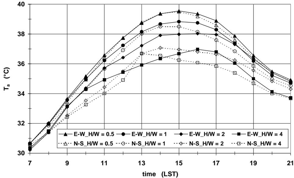
Figure 2 Diurnal variation of the simulated air temperature  $T_a$  at street level in urban canyons with aspect ratios  $H/W$  from 0.5 to 4 and for E-W and N-S orientations, typical summer day (1<sup>st</sup> August) in Ghardaia, Algeria (32.40° N, 3.80° E)
