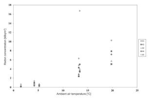
Fig. 3 Mean radon concentration as a function of mean surface air temperature
